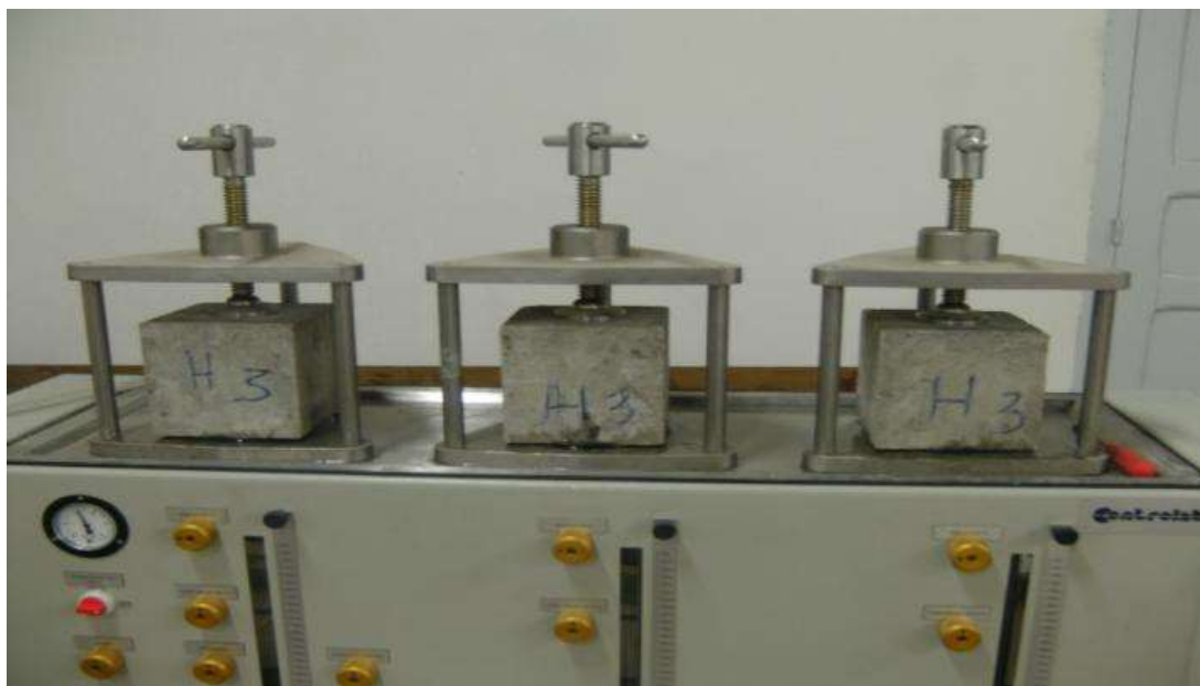
Fig. 4.13 Water Permeability Test
